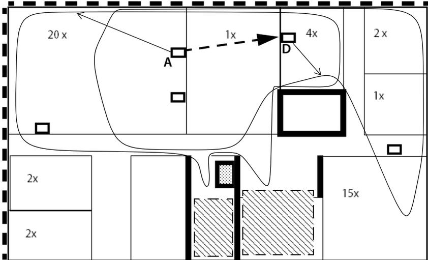
In the example, limitation lines are drawn for the wireless coverage for base stations A and D. The overlap areas are very good for both stations; synchronisation is also guaranteed between A and D. However, the measurement results of the other stations must be used to check whether a further base station is required in the shaded areas.
