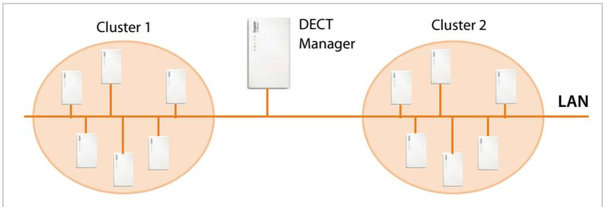
The DECT Manager is connected to the base stations and the PABX via the local network and is therefore not dependent on DECT ranges. This means that you can install separate DECT islands at your location but manage them centrally, i.e., they have access to the centrally configured IP connections, directories, etc.
